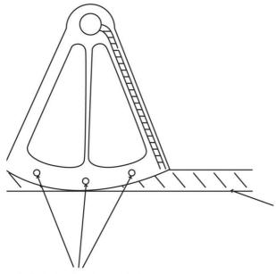
Handrail section to protect back of plate (ordered separately to plate)
