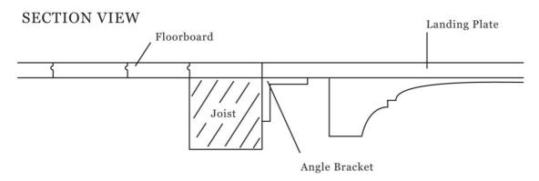
The Angle Brackets are supplied fixed to the landing, so they can be drilled and bolted to the finished floor joist
